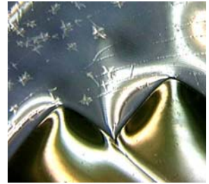
Cracks and splits after fusing.
