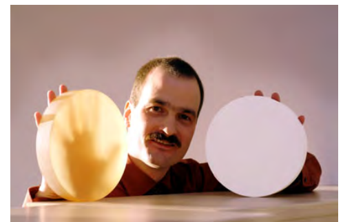
Material samples before and after transformation to the high temperature stability glass ceramic ZERODUR® K20
