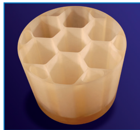
Rib thickness of 2 mm and pocket depths of 190 mm achieved on a 300 mm diameter demonstrator with standard diamond tool grinding
