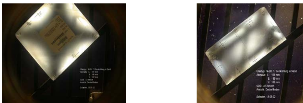
Figure 7: Breakdown of stress with cutting. Fine-annealed block of optical glass N-BK7 in crossed polarizers. Left: Original format L: 191 x W: 180 x H: 162 SBF: -13 nm/cm top-bottom. Right: After cutting in the middle L: 191 x W: 90 x H: 162 SBF: -4,5 nm/cm top-bottom. For large blanks such breakdown may not be expected since they are not cut.
