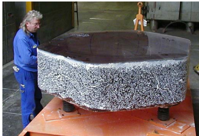
Figure 3: ZERODUR® near net shape raw casting
