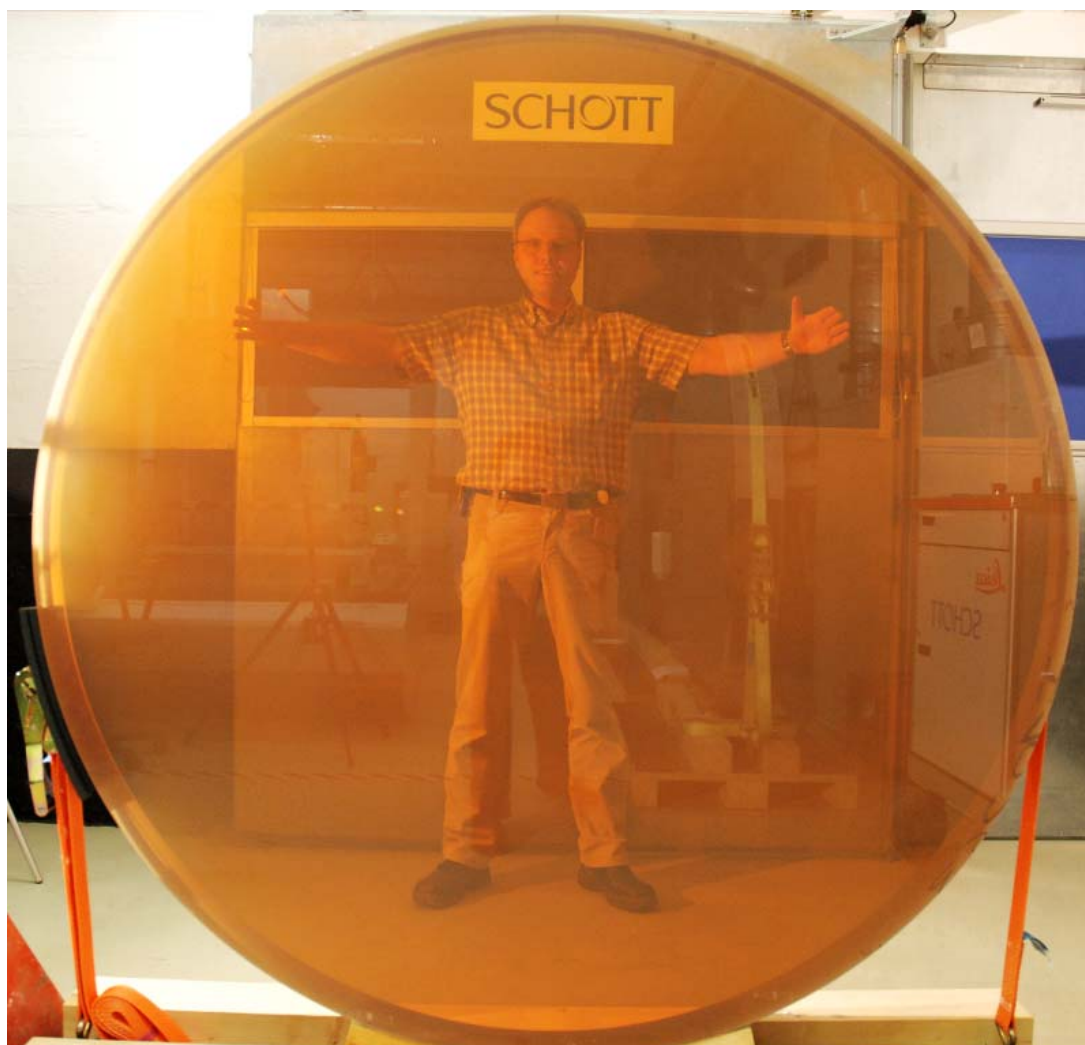
Figure 10: ZERODUR® blank with a diameter of 1.53 m a thickness of 176 mm and a weight of 819 kg, in optical standard grade striae quality and with excellent bubbles and inclusion quality.
