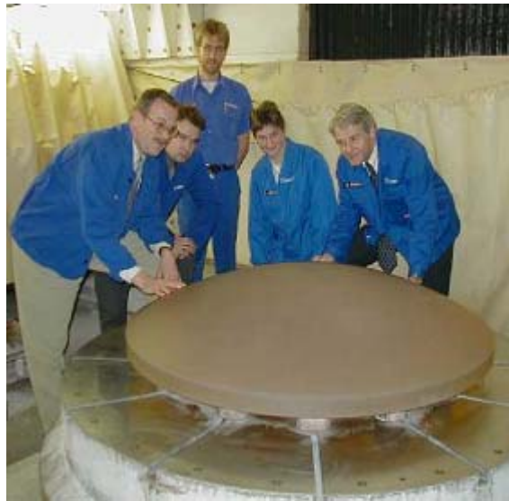
Figure 4: 1.33 m diameter ZERODUR® testing lens for the secondary mirror of GRANTECAN.
