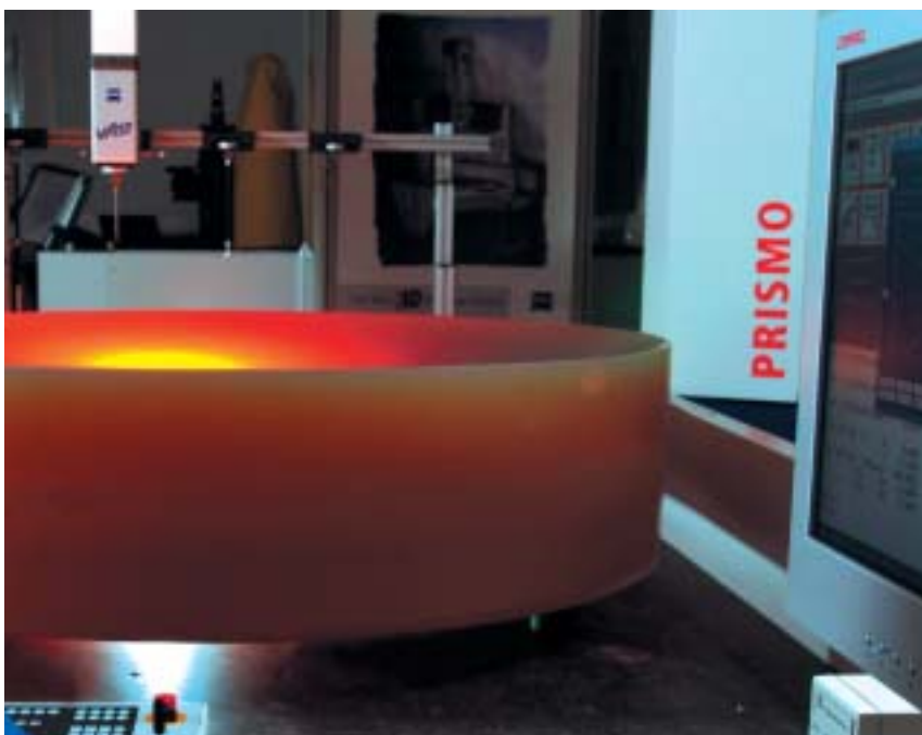
Modern coordinate measurement equipment in the final inspection of ZERODUR®
