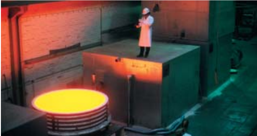
A 2-meter mirror blank casting is transported into the annealing furnace.
