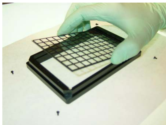
Optional Step 12: Remove microarray plate from tray for washing
