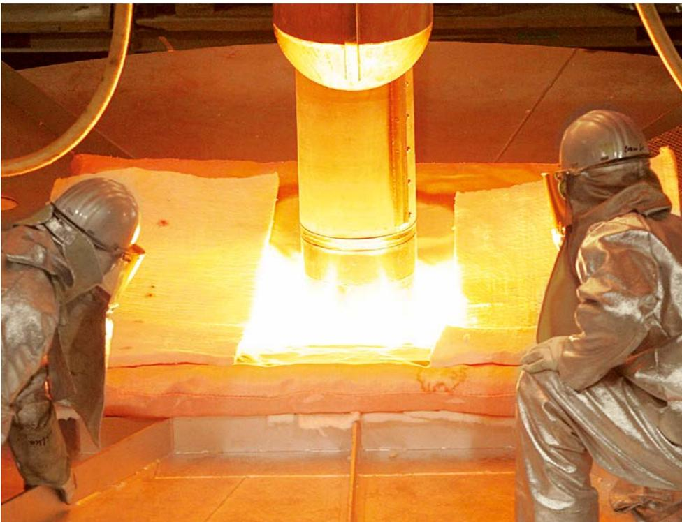
After a few months of hard work, SCHOTT Advanced Optics is excited to announce that we have completed the routine refurbishment of our ZERODUR® melting tank. This planned and scheduled maintenance is a routine part of the ZERODUR® production process, occurring every few years depending
