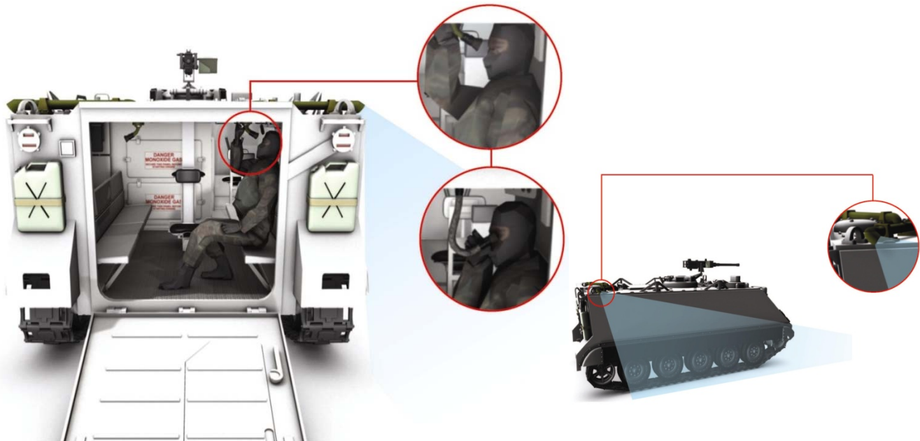
Sample application of remote viewing through a SCHOTT Wound Image Bundle.
