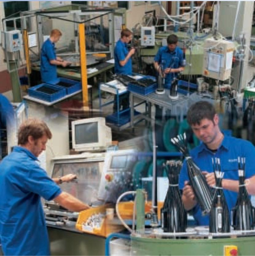
*The fiber optic light guides for the BMW 5 series lighting system are manufactured at Schott Fiber Optics in Doncaster, England: 10,000 pieces per week.*
