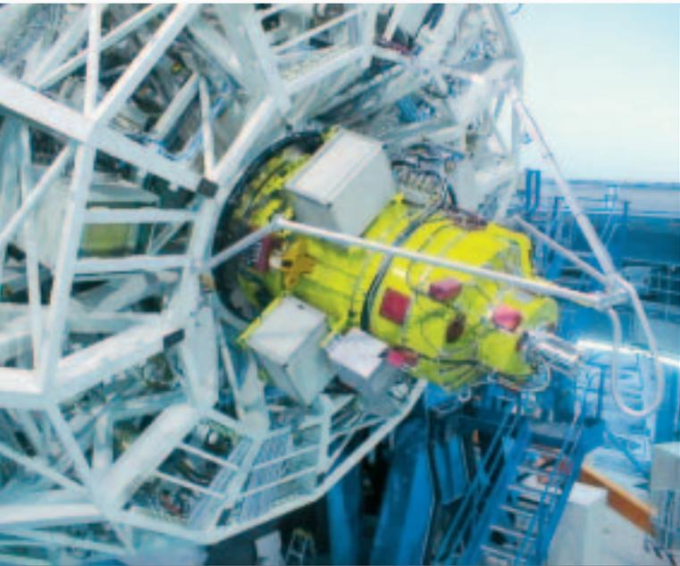
The VLT instrument FORS1 is flanged on to a support element of the main mirror. The imaging optics, made of special glasses from Schott, are located in the yellow cylinder. The silver and red boxes contain the electronic components and the servomotors for the control system.
