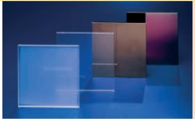
flächenmodifikation = Institute for Surface Modification of Leipzig), is investigating various correction processes to further improve the overall surface of the masks by carefully removing the minutest amounts of material from it.
