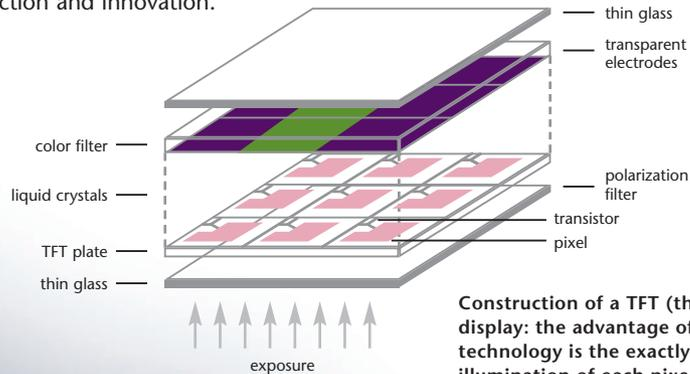
**Construction of a TFT (thin film transistor) display: the advantage of this display technology is the exactly triggered illumination of each pixel by a transistor. Millions of pixels on large-format displays allow an outstanding brilliance and a high contrast of the reproduced image.**
