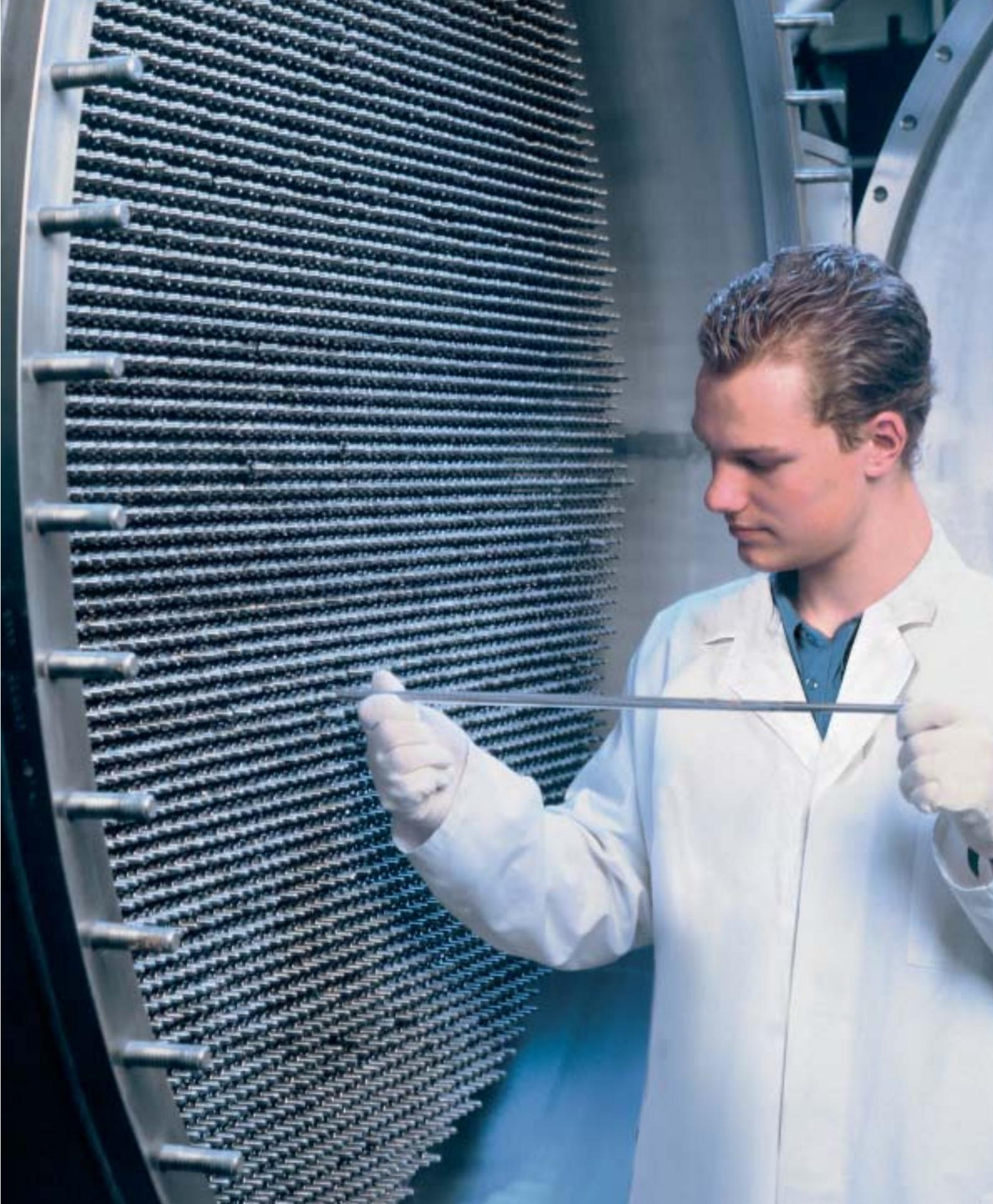
Three separate generators each with some 21,000 "Duran" glass tubes – 10,324 at each end – were installed in the world's largest ozone production system at VCP in Brazil. The outer and inner diameters of the special glass tubing required for the construction of the electrodes have an extremely narrow range of permissible variation.
