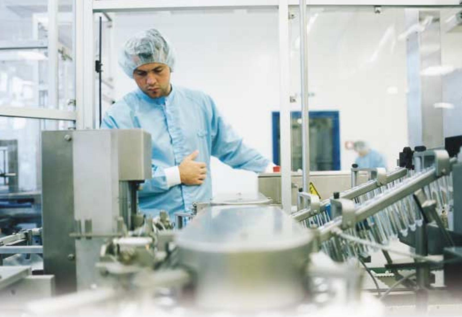
The plastic syringes are injection-molded in a clean room, sterilized, packed in special trays and, as a particular service, delivered directly to the customer's clean room ready to be filled.
