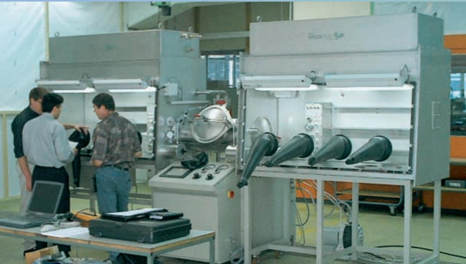
*Equipment for the investigation and use of the new technology. The processes are carried out under clean room conditions and in an inert gas atmosphere.*
