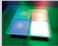
An OLED consists of a substrate, a transparent electrode, one or more thin organic layers and a counter-electrode.
