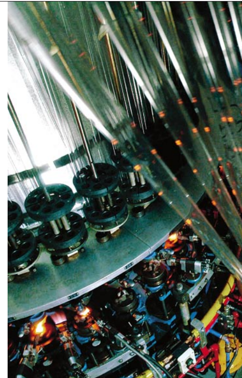
Fiolax® glass tubing is used to make advanced pharmaceutical packaging. SCHOTT-Rohrglas GmbH is the world's first tubing company to be certified according to ISO 15378.
