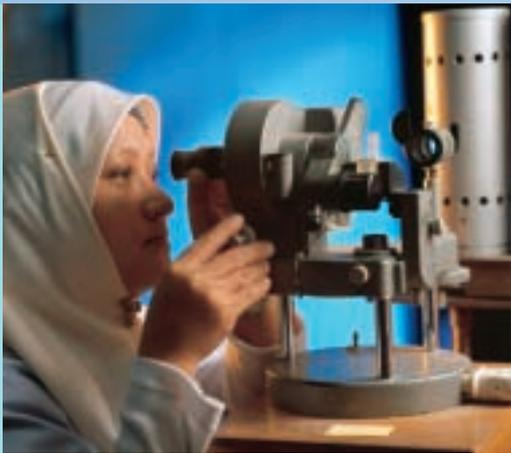
*Digital projection calls for maximum precision in determining refractive index.*
