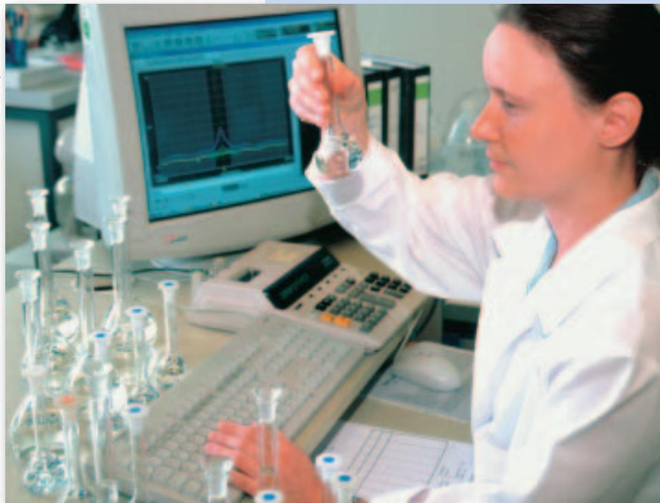
The classic wet-chemical analysis is indispensable: measuring samples with inductively coupled plasma optical emission spectroscopy (ICP-OES).
