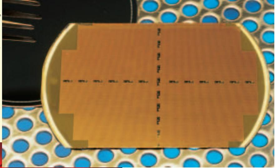
Using the molecular epitaxy process, many layers are crystallized onto substrates made from gallium arsenide. These act as reflectors on laser diodes or as active amplifiers of light.
