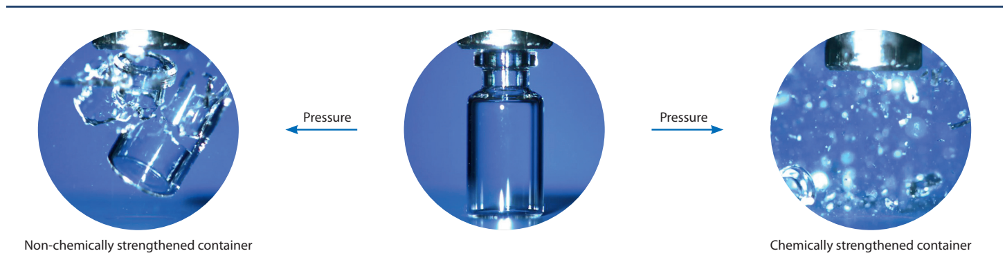
Figure 2 Breakage behavior of a non-strengthened (left) and chemically strengthened (right) glass container upon axial compression acc. to DIN EN ISO 8113 (Glass containers – Resistance to vertical load — Test method ISO 8113:2004)
