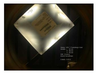
Figure 8: N-BK7 block with internal stress.
