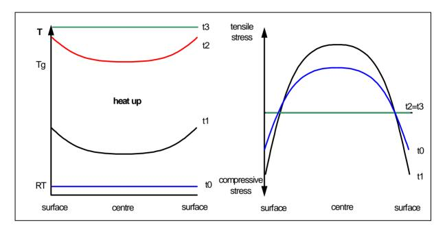
**Figure 4**: Schematic representation of the stress inside a glass as a function of the temperature distribution after different times for a constant heating rate.
