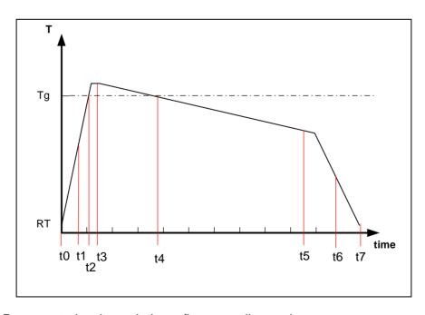
Figure 3: Representative times during a fine annealing cycle.
