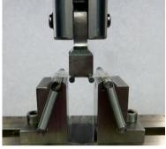
**Figure 5:** Four-point bending setup.
