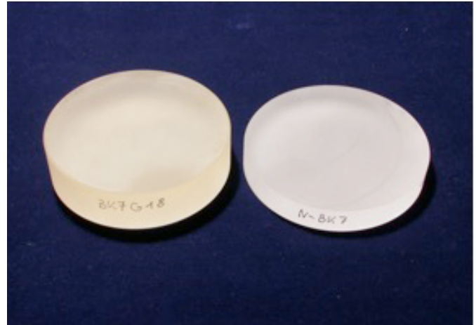
Fig. 3-1: Cerium stabilized BK7G18 and non stabilized N-BK7 in direct visual comparison.
