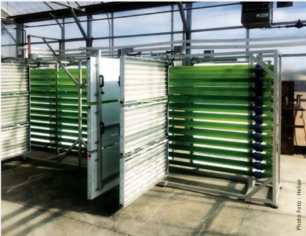
The Arizona Center for Algae Technology and Innovation is equipped with a Heliae Helix™ seed production photobioreactor with optional light panels.
